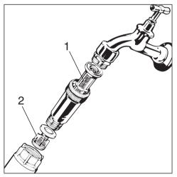
Clean the large area filter (1) and the fine filter (2) or replace if necessary.
